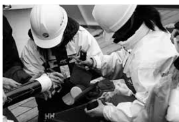
船上での海底堆積物処理風景 Sub-sampling of the sediment core on the deck of the research vessel
